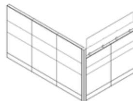
**2** Insert the screen into the mounts and secure with screws
