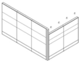
**1** Attach desktop mounts to the top of the panels where the screen will go.
