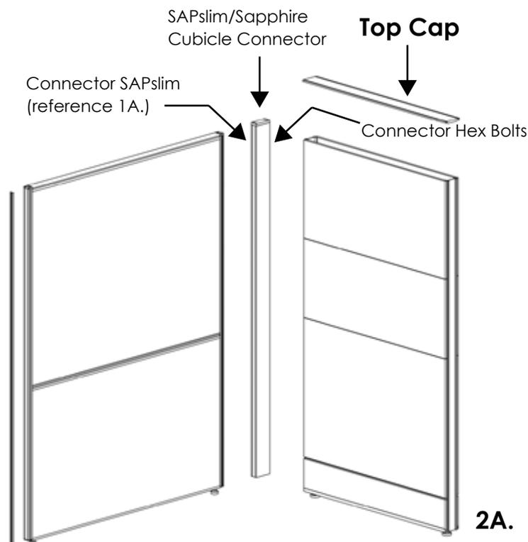
2. Sapphire Cubicle panel attaches to connector by using a washer and hex bolt. (figure 2B.).
