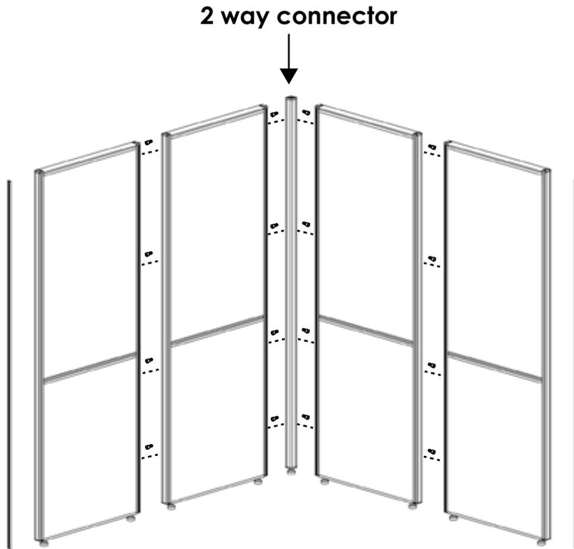
Connect the panels to the connector first and then attach second set of panels.
